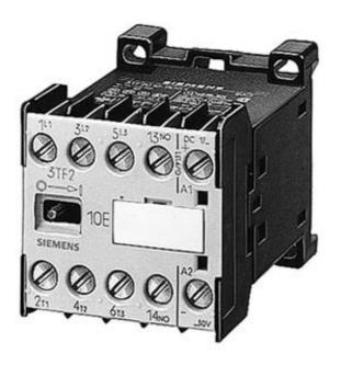
CONTACTOR SIZE 00 3-POLE AC-3 4KW/400V, PIN, PLUG CON. 6.3 MM, FOR SIMODRIVE AUX. SWITCH 02 E (1NC) WIDTH 90 MM DC MAGNET SYSTEM, 0.97...1.1 US 24 V DC
