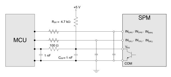
Figure 9. Recommended MCU I/O Interface Circuit
