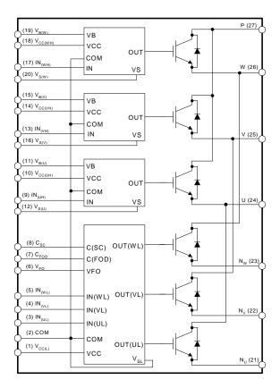
Figure 3. Internal Block Diagram
