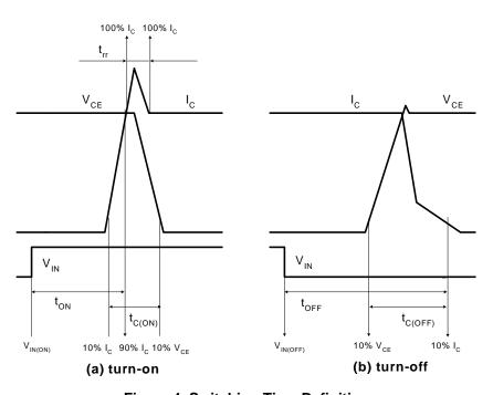
Figure 4. Switching Time Definition
