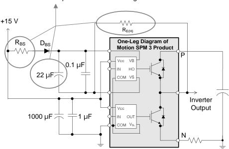
Figure 10. Recommended Bootstrap Operation Circuit and Parameters
