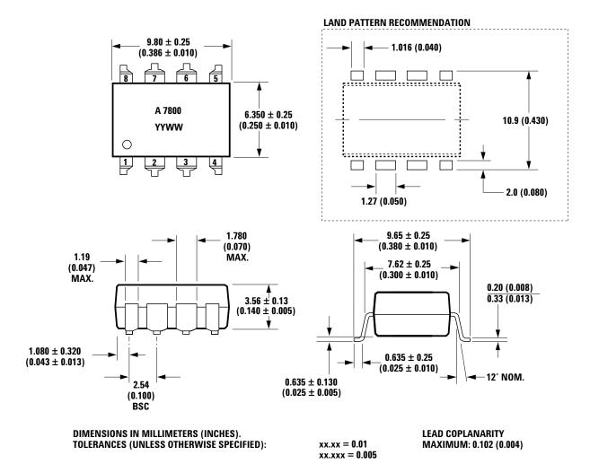
NOTE: FLOATING LEAD PROTRUSION IS 0.5 mm (20 mils) MAX.
