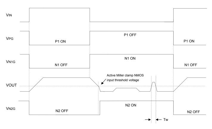
Active Miller effect clamp NMOS keeps turn-on if  $T_{\rm W}$  does not exceed active Miller clamp NMOS filter time
