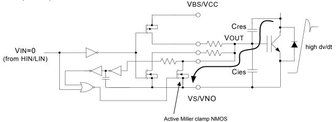
When HIN/LIN is at low level and the voltage of the VOUT (IGBT gate voltage) is below active Miller effect clamp NMOS input threshold voltage, the active Miller effect clamp NMOS is being turned on and opens a low resistive path for the Miller current through Cres.
