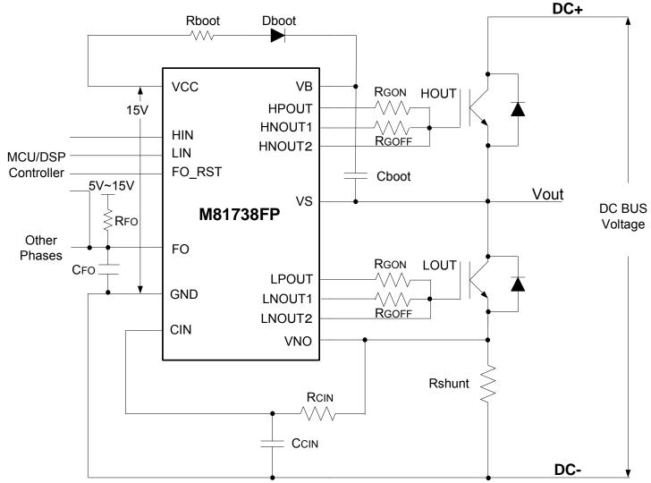
Note: If HVIC is working in high noise environment, it is recommended to connect a 1nF ceramic capacitor to FO pin.
