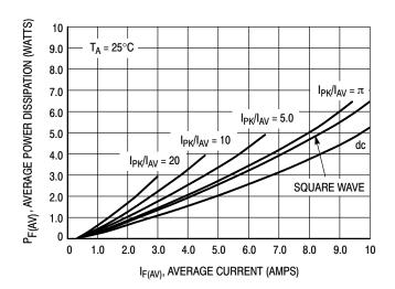
Figure 5. Forward Power Dissipation
