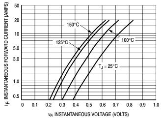
Figure 1. Typical Forward Voltage
