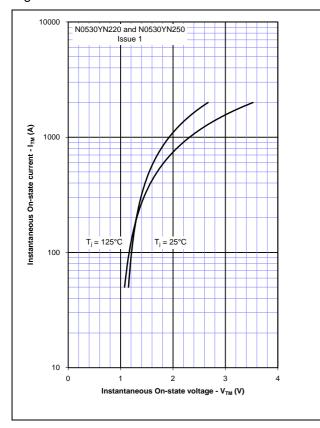
Figure 1 – On-state characteristics of Limit device
