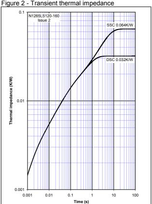
Figure 2 - Transient thermal impedance
