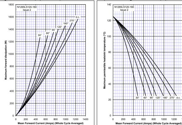
Figure 16 - On-state current vs. Heatsink temperature - Single Side Cooled (Square wave)
