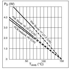
Figure 14. Allowable power dissipation vs. ambient temperature.
