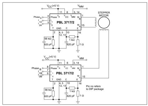
Figure 8. Typical stepper motor driver application with PBL 3717/2.
