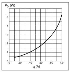
Figure 13. Typical power dissipation vs. motor current.
