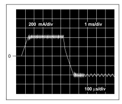
Figure 5. Motor current  $(I_{\rm M})$ , Vertical : 200 mA/div, Horizontal: 1 ms/div, expanded part 100  $\mu$ s/div.
