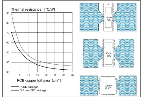
Figure 16. Copper foil used as a heatsink.
