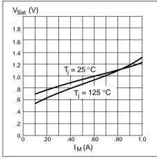
Figure 10. Typical sink saturation vs. output current.
