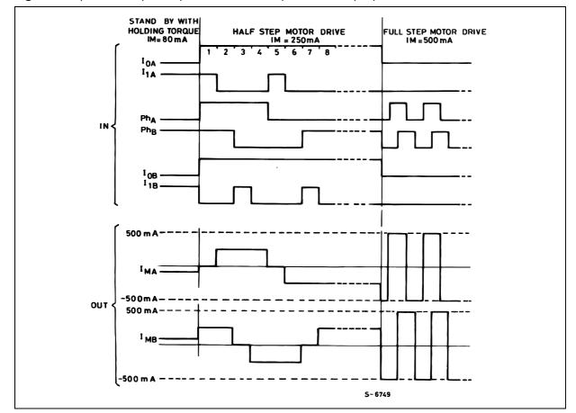
Figure 5: Input and Output Sequences for Half Step and Full Step Operation
