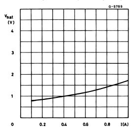
Figure 8 : Sink Saturation Voltage versus Output Current
