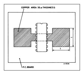
The diagram of fig. 11 shows the maximum dissipable power  $P_{tot}$  and the  $R_{th j-amb}$  as a function of the side " $\alpha$ " of two equal square copper areas having a thichkness of  $35\mu$  (see fig. 10).
