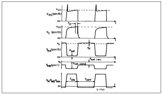
Figure 3: Two Phase Bipolar Stepper Motor Driver
