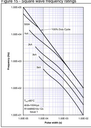
Figure 16 - Square wave frequency ratings
