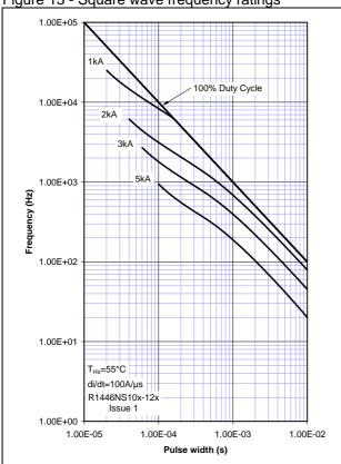
Figure 14 - Square wave frequency ratings
