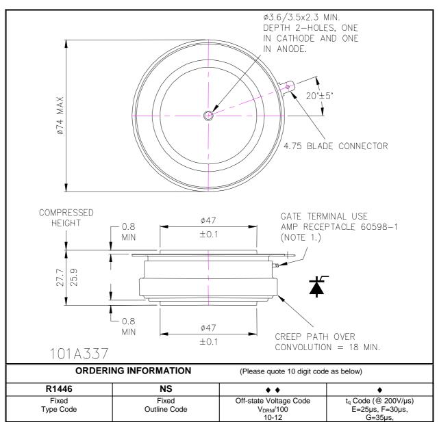
Typical order code: R1446NS12F – 1200V V<sub>DRM</sub>, 30µs t<sub>q</sub>, 27.7mm clamp height capsule.
