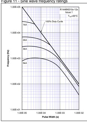
Figure 12 - Sine wave frequency ratings
