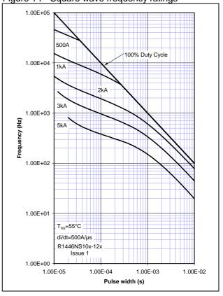
Figure 15 - Square wave frequency ratings
