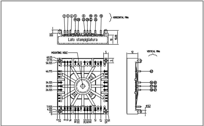
Case T74 (Suggested hole diameter for the solder pins in the circuit board: 2mm. Suggested hole diameter for the mounting pins in the circuit board: 3,6mm )
