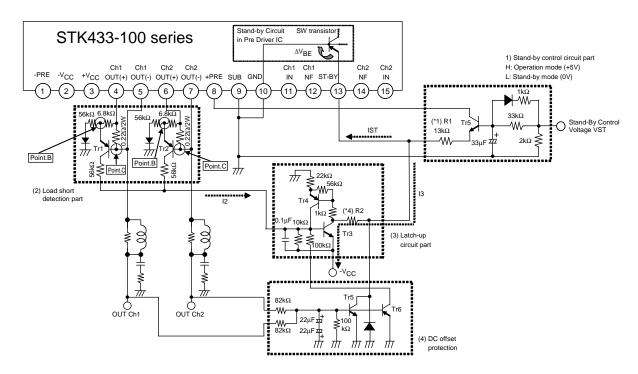
The protection circuit application for the STK433-100sr consists of the following blocks (blocks (1) to (4)).
